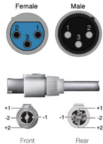
Figure 9. Cannon® XLR and Neutrik® SpeakOn connectors
